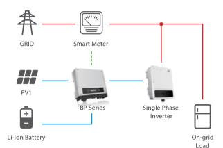
O2 System Upgrading Design for Single Phase & Dual MPPT Inverters
