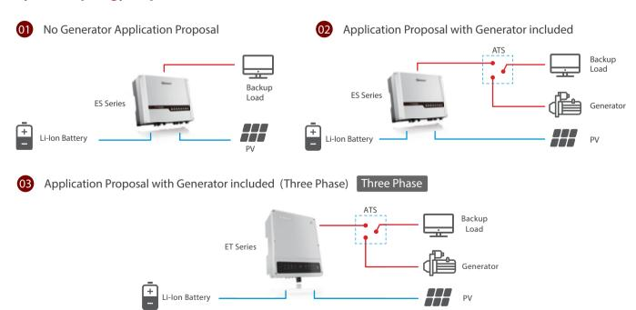
Incase of insufficient battery & PV supply without public grid, a generator could be adopted automatically or manually switch supply from hybrid back-up side to supply from generator
