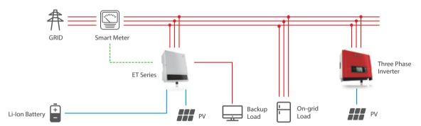
ET hybrid system capacity could be extended by connecting with a 3-phase grid-tie solar system, especially for big battery capacity. The ET Series reduce the power loss from PV side by using exclusively the energy from the 3-phase grid-tied solar system (anti-reverse system). Power from grid-tied system may support the loads together with ET hybrid system, while battery charging, before it could feed into grid.
